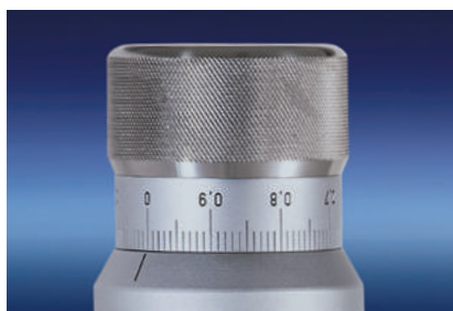
The lifting ring depth adjustment of the DS 8 knife holder
